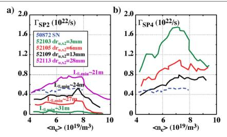
**Figure 6.** Ion currents to (a) SP2 (lower primary inner-wall strike point) and (b) SP4 (outermost secondary strike point) for density ramps in LFS SF – configurations for varying X-point separation  $dr_{u,x2}$ . (Reproduced with permission from [16].)
