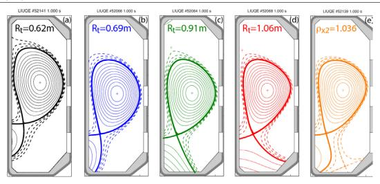
**Figure 4.** Flux-surface contours of TCV equilibria for (a)–(d) varying major radius of the outer strike point, up to the super-X case, (e) X-point-target divertor. (Reproduced with permission from [17].)
