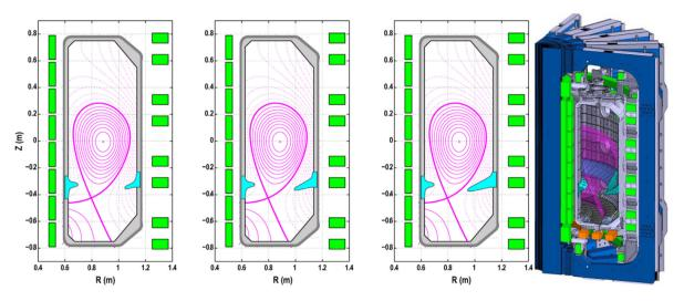
**Figure 11.** (Left) Sketches of baffles for varying divertor closure, limiting the SOL at the flux surface with an outboard midplane separatrix separation of ~1 cm, 2 cm, and 3 cm, respectively, with centered X-point. (Right) 3D view for the case with the longest baffles. (Reproduced with permission from [4].)
