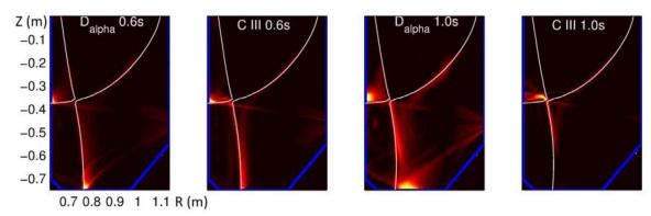
Figure 5.  $D_{\alpha}$  and C III emissivity profiles 0.4s before and at the onset of detachment (occurring at 1.0s). (Reprinted from [22], Copyright 2016, with permission from Elsevier.)
