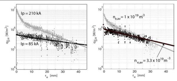
Figure 7. Profiles of parallel heat flux to the target mapped to the outboard midplane in inboard limited plasmas for (left) two current values at line-averaged density  $1.7 \times 10^{19}$  m<sup>-3</sup> and (right) two density values at a plasma current of 140 kA. (Reproduced with permission from [28].)
