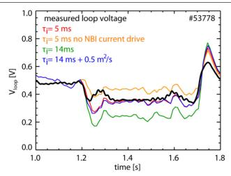
**Figure 2.** Measured loop voltage versus value predicted by TRANSP with different ion confinement time values, also in a case with suppressed NBCD and a case with ad hoc turbulent diffusion. (Reproduced with permission from [8].)
