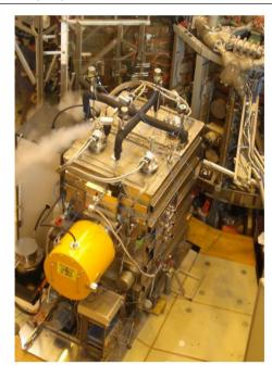
**Figure 1.** The neutral beam injector of TCV.
