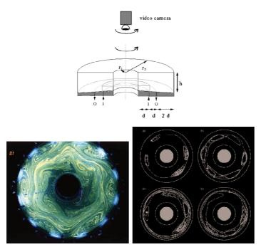
Fig. 11. (a) Rotating annulus. (b) The formation of eddies inside the rotating annulus, as recorded by the camera (left panel), and (c) typical orbits of tracer particles inside the annulus (right panel).
