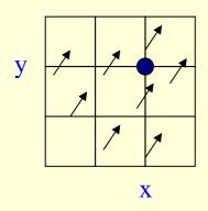
All fluid properties are measured with respect to a *fixed coordinate system*. Time variations are described by *local derivatives* at a given coordinate location, e.g.
