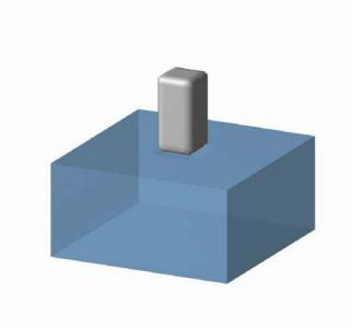
Water clashing over a ship's deck with a rectangular obstacle.
