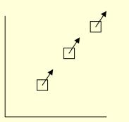
All fluid properties are measured with respect to a *moving control mass* of variable volume V(t) occupied by the same particles at all times. Time variations are described by *total derivatives* at the location of the control mass, e.g.
