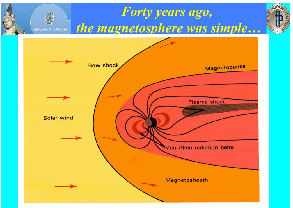
Lai Figure 1—Earth's magnetosphere. The sketch shows important features of the plasmas and waves in the magnetic fields that surround Earth. (Lanzerotti and Krimigis, Physics Today, 1985)
