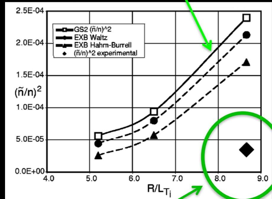
Experimental low-k ( $k_{\theta}\rho_s < 0.5$ ) density fluctuation level
