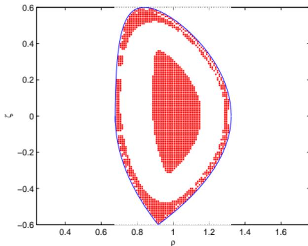
*The stability function  $A$  for a state with  $\alpha = 15$  and  $M_0^2 = 0.02$ . The red coloured region is where the sufficient condition  $A \geq 0$  is satisfied*
