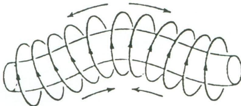
*The kink instability is associated with a bending of the plasma column (z-pinch).*
