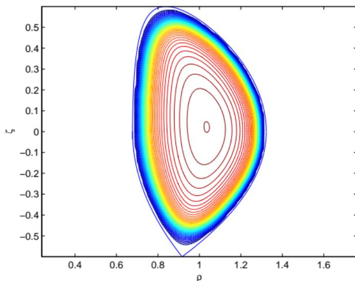
*Equilibrium with ITER-like elongation,  $\kappa = 1.86$ , triangularity,  $\delta = 0.5$ , and parallel flow constructed numerically by imposing analytically the boundary.*
