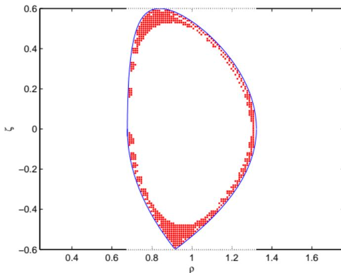
*The stability function  $A$  for a state with  $\alpha = 10$  and  $M_0^2 = 0.005$ . The red coloured region is where the sufficient condition  $A \geq 0$  is satisfied.*
