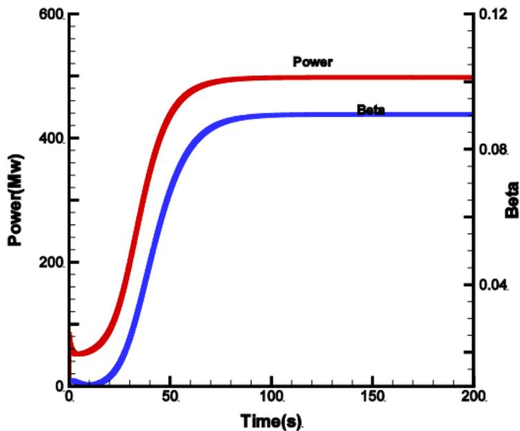
*Neutron generated power and beta as functions of time.*
