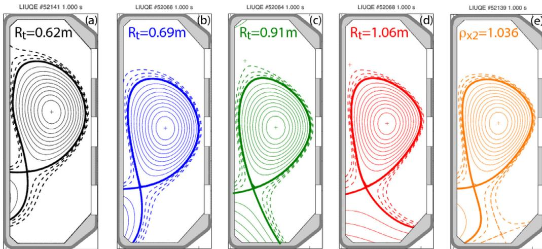
**Figure 4.** Flux-surface contours of TCV equilibria for (a)–(d) varying major radius of the outer strike point, up to the super-X case, (e) X-point-target divertor. (Reproduced with permission from [17].)
