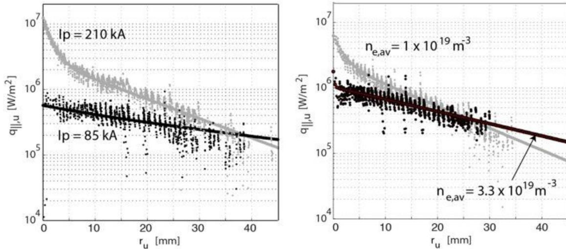
**Figure 7.** Profiles of parallel heat flux to the target mapped to the outboard midplane in inboard limited plasmas for (left) two current values at line-averaged density  $1.7 \times 10^{19} \text{ m}^{-3}$  and (right) two density values at a plasma current of 140 kA. (Reproduced with permission from [28].)
