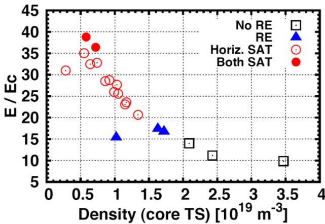
**Figure 8.** Classification of runaway-electron discharges versus central density and normalized toroidal electric field, based on signals from heavily shielded HXR detectors: no RE = no signal, RE = finite signal, Horiz. SAT = midplane detector saturated, Both SAT = midplane and top detectors saturated. (Reproduced with permission from [36].)
