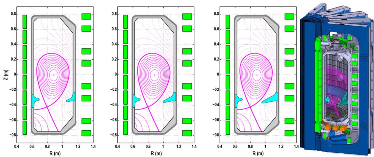
**Figure 11.** (Left) Sketches of baffles for varying divertor closure, limiting the SOL at the flux surface with an outboard midplane separatrix separation of  $\sim 1$  cm, 2 cm, and 3 cm, respectively, with centered X-point. (Right) 3D view for the case with the longest baffles. (Reproduced with permission from [4].)
