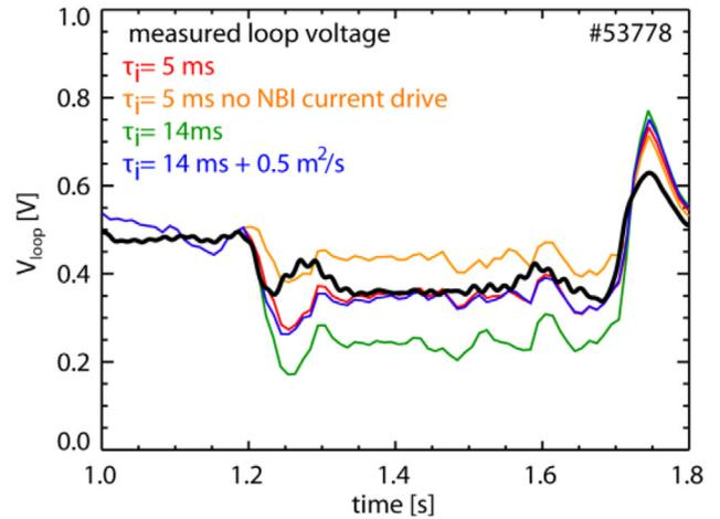
Figure 2. Measured loop voltage versus value predicted by TRANSP with different ion confinement time values, also in a case with suppressed NBCD and a case with ad hoc turbulent diffusion. (Reproduced with permission from [8].)
