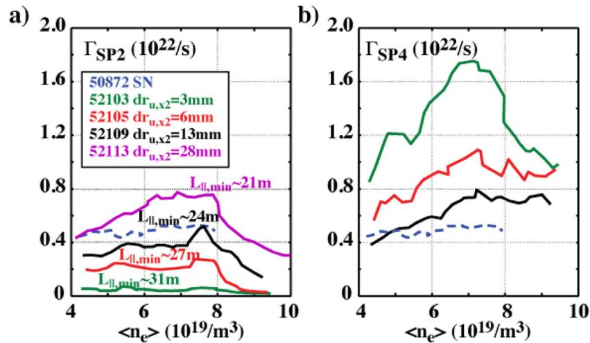
**Figure 6.** Ion currents to (a) SP2 (lower primary inner-wall strike point) and (b) SP4 (outermost secondary strike point) for density ramps in LFS SF – configurations for varying X-point separation  $dr_{u,x2}$ . (Reproduced with permission from [16].)
