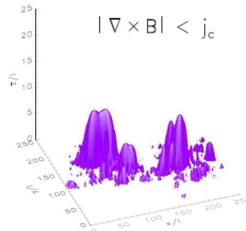
We use here the twist threshold (left,  $\hat{\mathbf{b}} = \mathbf{B}/|\mathbf{B}|$ ), motivated by Parker's critical angle. Our  $u_c$  corresponds to a twist scale  $1/u_c \sim 3000$  km. Inside the violet regions,  $\eta > 0$  and  $\mathbf{E} = \eta \mathbf{j}$  exceeds  $E_D$  by about one magnitude. By the force-free assumption  $\mathbf{j} = \alpha \mathbf{B}$  with  $\alpha > 0$ ,  $\mathbf{E}$  is *parallel*.
