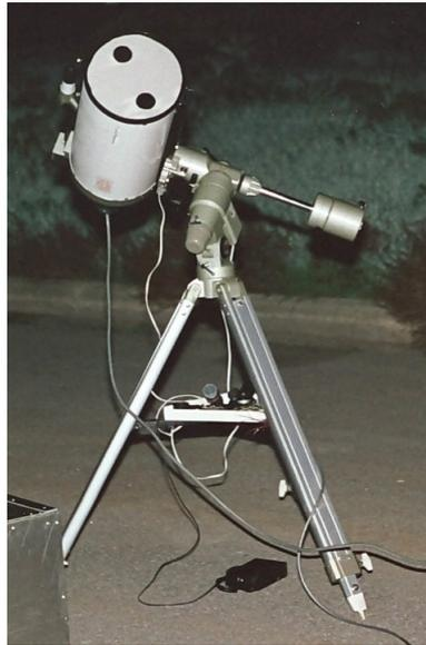
Figure 6.1: The Vixen Telescope Along with the ST4 CCD Camera.
