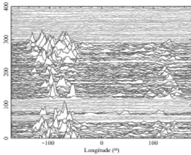
This illustration shows several nulls in light gray and a transition to a weak mode interval lasting several thousand pulses, starting at pulse number 300.
