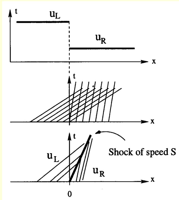
The characteristics cross, forming a *shock wave*.
