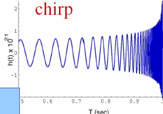
$$f_{\text{BH}} \sim 12 \text{kHz} \left( \frac{1 M_\odot}{M} \right)$$
