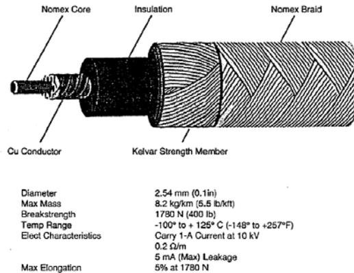
Fig. 3. Construction of the TSS tether.
