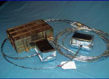
Flux Gate magnetometer  $\Rightarrow$  magnetic field data up to  $\sim 1\text{Hz}$
